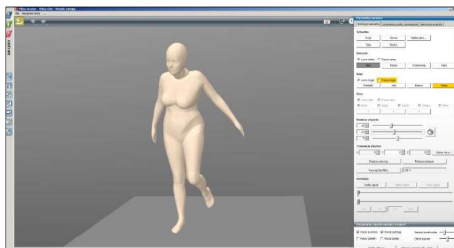
Rys. 2. Awatar w systemie CAD ASSYST: tworzenie ruchu awatara [źródło: Vidya 3D CAD ASSYST, education version 20.13]
